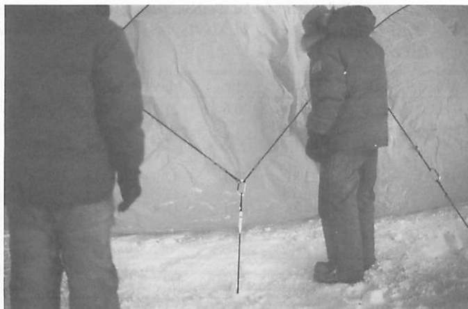
Fig. 3. Buried anchors with ropes. The guy ropes connected to the anchor ropes with carabiners keep the shape of the dome.
