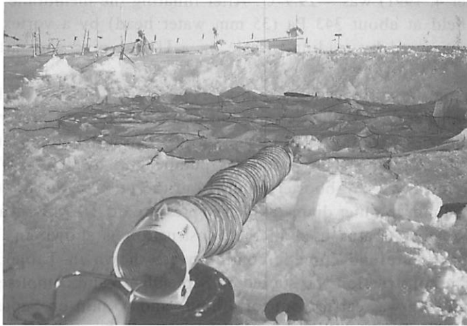
Fig. 5. Spread membrane bag with ventilator.
