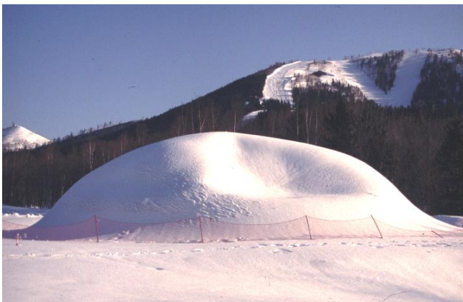
Fig. 6 Large creep deformation before collapse
